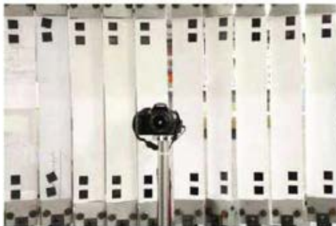
Figure 5.2 Example photo for the optical analysis of the elongation of the strips
